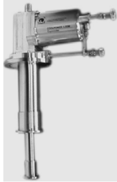
Figure 12. COOLPOWER 4.2 GM Cryocooler allows for cooling the samples down to 20 K in approximately 90 minutes. Figure is from (Leybold, 2012).
