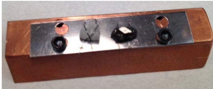
Figure 10. \text{ThO}_2 and another sample mounted on a thin tantalum sheet by arc welding tantalum wires to secure the samples. The configuration is then secured onto the OFHC ^{101}\text{Cu} sample holder of 1'' \times 0.375'' \times 0.375'' (length \times width \times height).
